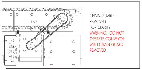
WARNING: To check drive sprocket tension, shut "OFF" and lock out power source before any adjustments are attempted.
